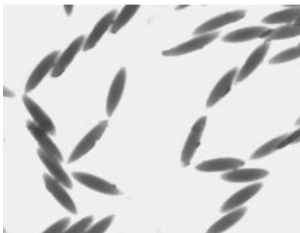
Figure 12 Transmission electron micrograph of 1 \mu\text{m} polystyrene ellipsoids and magnetite particles.
